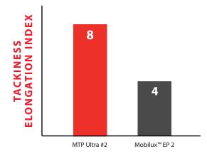
Elongation is a measure of the adhesive-cohesive "stringiness" of a grease and indicates its ability to effectively travel through moving systems and create a protective coating.
